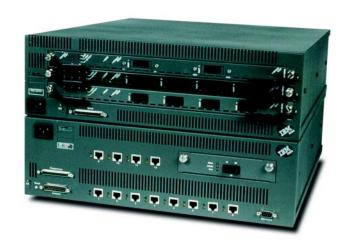
The IBM 8285 Nways® ATM Workgroup Switch is a multipurpose, expandable ATM switch that simplifies ATM implementation. It has twelve 25-Mbps ATM ports for desktop or server connections and a feature slot for optional 155-Mbps I/O cards for connecting to a server or another switch. I/O cards for 155-Mbps ATM on multimode fiber (MMF) and single-mode fiber (SMF) are supported.
