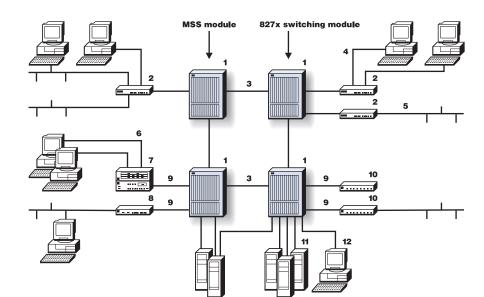
**Solution:** Fast Ethernet modules in the 8260 with Packet Channel-to-ATM connectivity allow Fast Ethernet servers or Ethernet switches with Fast Ethernet uplinks transparent connectivity to ATM and Multiprotocol Switched Services (MSS).
