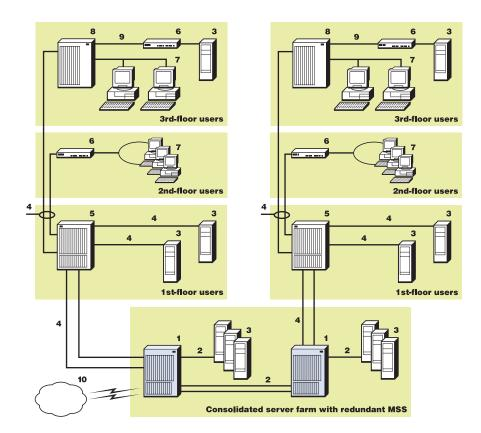
**Solution:** The 8265 Nways ATM switch provides the nonblocking 155-Mbps and 622-Mbps port density and 12.8 Gbps of cell-switching capacity necessary for today's ATM backbone networks. It is also the perfect solution for ATM-attached server farms and concentration of large numbers of LAN switching edge devices with 155-Mbps ATM uplinks.
