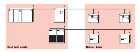
**Solution:** The 2218 supports the consolidation of the multiple serial protocols typically found in a branch-bank network over a common Frame Relay connection.
