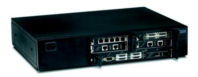
The IBM 2212 Access Utility is a branch office in a box. The IBM 2212 Access Utility makes it easy to connect local area networks (LANs) to the mobile workforce, and remote LANs or branch offices using advanced multiprotocol virtual private networks (VPNs), for access to the Internet and company backbone. The IBM 2212 Access Utility provides both cost-effective computing across a broad range of remote locations, as well as the flexibility to grow in meeting tomorrow's networking needs.
