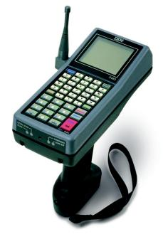
The 2483 Integrated Laser PTC is a battery-powered, hand-held data collection RF device with an integrated bar-code laser scanner. The LCD can show up to 16 lines of information, each line up to 21 characters long. Data can be entered into host system applications using the 2483 PTC via the integrated bar-code laser scanner or through the PTC keypad. The three models of the 2483 PTC indicate the range of the integrated bar-code laser scanner.
