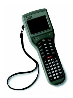
The IBM 2486 Portable Transaction Computer (PTC) is a compact, full-function, battery-powered, hand-held RF wireless computer used to collect, store and transmit data. Its design features a 2.4-GHz DSSS radio and an integrated laser scanner angled down 20 degrees, facilitating scanning with minimum movement.
