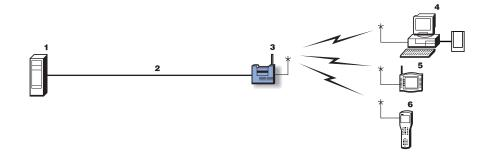
**Solution 2:** Configure an IBM 2488 Pen-Based system (Model 300 or 800) with a wide area radio (ARDIS, CDPD, RAM Mobitex, etc.) and establish an account with a wireless service provider. From anywhere within the service area, the IBM 2488 would be able to establish a connection to any host system attached to the service provider as either a client device or in a file transfer mode.
