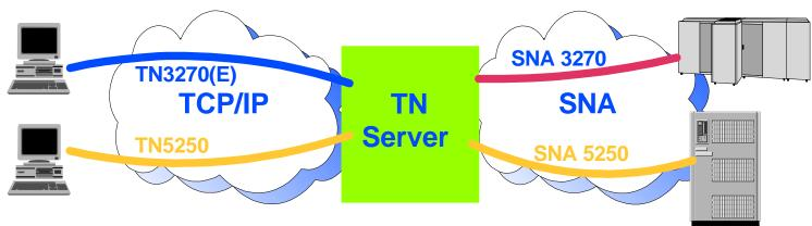
Gateway that enables clients and workstations on a TCP/IP network to access applications in an SNA network
