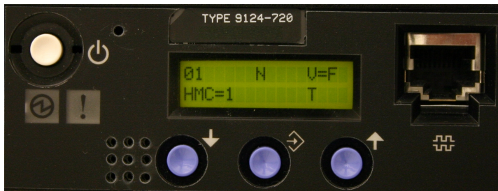
Illustration 18: LCD control panel of a managed system that has communication with an HMC
