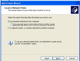
You can also select [Network Printer] but select [Local Printer] here even if you use a printer by connecting to a network.
