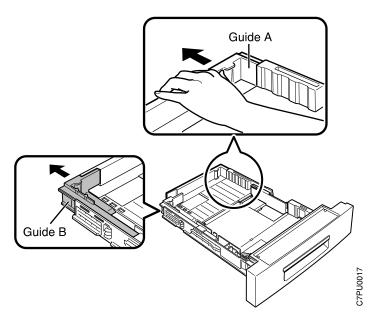
c. To shorten the tray, slide guide B in to the edge of the paper. Then slide guide A in to align with B or until it hits the stop.
