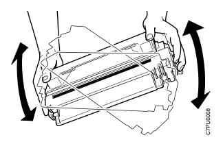
6. Place the cartridge on a flat surface and locate the yellow tape at the end of the cartridge. Pull the end of the tape straight out to remove the toner seal.
