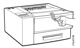
Press the button on the top of the printer to open the top cover.
