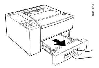
2. Press down on the bottom plate of the paper tray until it snaps into position.
