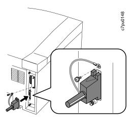
3. Attach the other end of the cable into the parallel interface slot on your PC or workstation.
