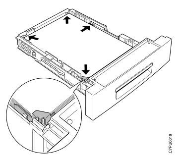
5. If the paper is narrower than the tray, adjust the side guide so that it presses lightly against the side of the paper stack.
