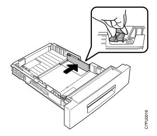
b. To lengthen the tray, slide guide A out. Then slide guide B to align it with guide A.
