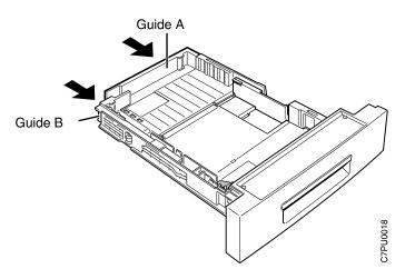
4. Insert the paper into the tray. Make sure you place the corners of the paper under the retaining clip at the front of the tray and the plastic tabs on the end and side of the tray.
