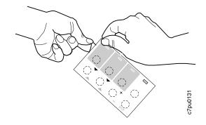
5. Position the template so that the top of the template lines up squarely with the top of the operator panel. Working down from the top of the template, gently press it into place.
