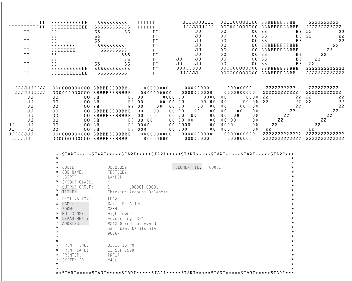
Figure 26. Sample Header Page. Additional distribution information is produced by the default APSUX01 exit supplied with PSF.
