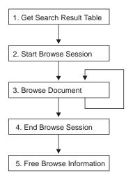
Figure 18. Sequence of API functions—using the Text Extender sample browser
