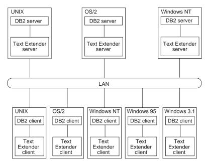
Figure 1. Integration of Text Extender into the DB2 client/server environment
