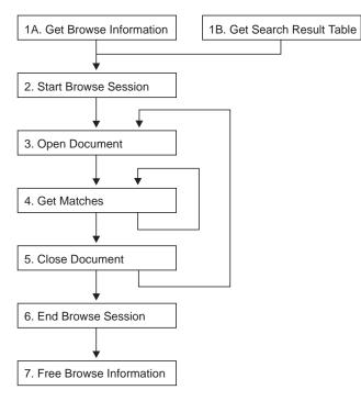
Figure 16. Sequence for using the API functions
