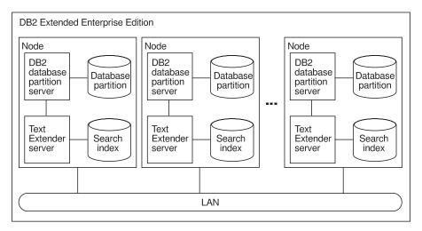
Figure 3. Integration of Text Extender into the DB2 partitioned database environment
