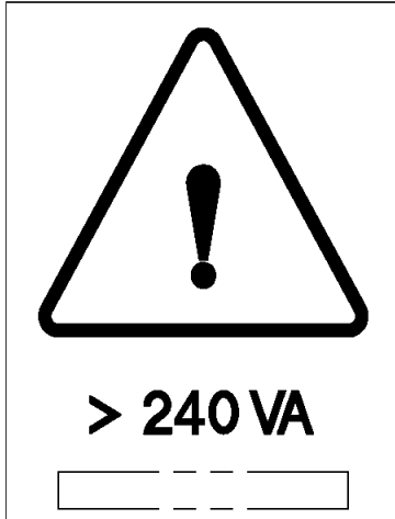
Figure 4-5. Safety Label—Power Distribution Unit DC Section
