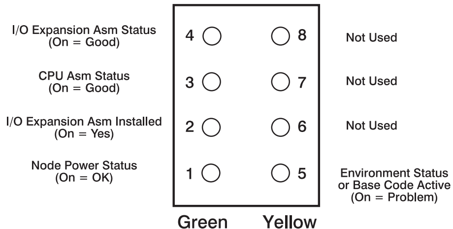
Figure 1-5. 332 MHz SMP Node Supervisor Card LEDs
