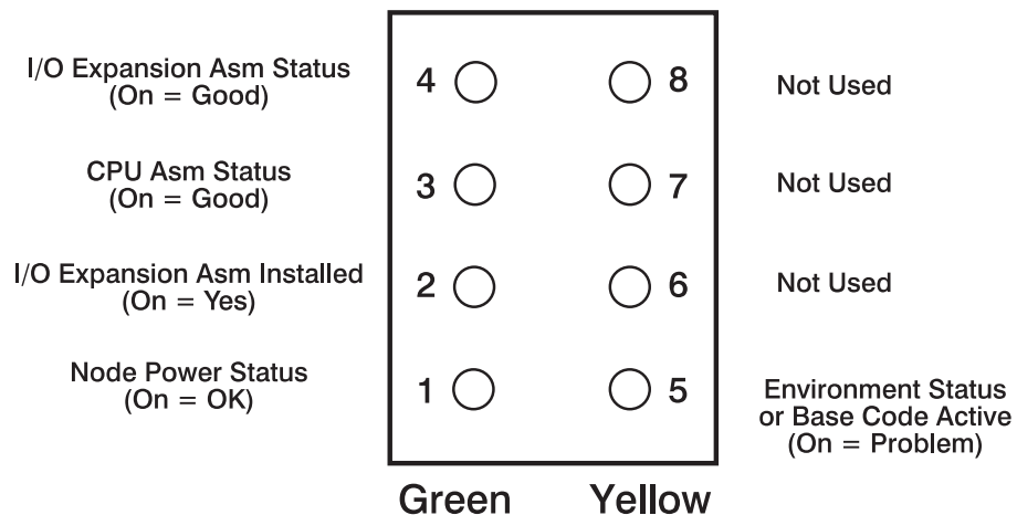
Figure 1-6. POWER3 SMP Node Supervisor Card LEDs
