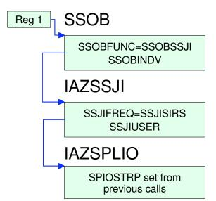
Register 1 points to SSOB SSOBINDV points to SSJI SSJIUSER points to IAZSPLIO
