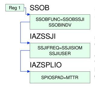
Register 1 points to SSOB SSOBINDV points to SSJI SSJIUSER points to IAZSPLIO
