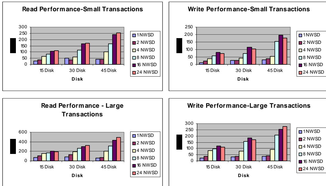
Figure 4 The figures above show read and write performance for small (4k-64k) and large transactions (128k+). This experiment shows that adding disk drives increases the throughput. A system with 45 disk drives will be able to transfer approximately 3 times faster than a system with 15 disk drives. Notice 24-network storage descriptions were used in order to achieve maximum performance.
