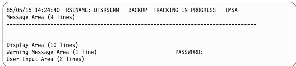
Figure 2. Master terminal format in XRF environment
