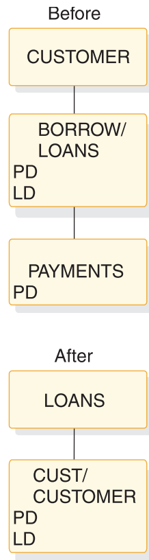
Figure 153. Logical child, physical pairing—virtual delete rule example: before and after
