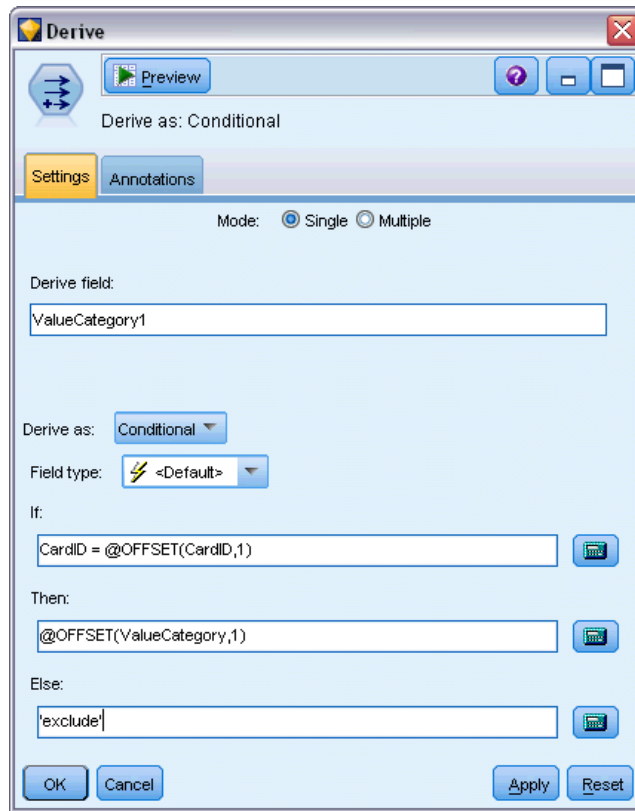
Figure 7-3 Conditional Derive comparing values of one field to those of the field before it
