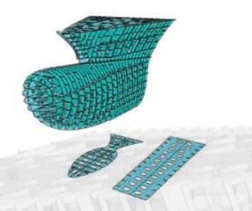
Not all structural details are standard so the solution provides efficient interactive tools to create individual details that still carry the full spec-driven implementation. Once again, copy and paste interactions allow designers to re-use and interactively adapt design detailing.
