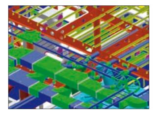
To support construction by zones, trays and hangers can be structured within the same assembly structure as the physical parts. This enables higher levels of supplier coordination, component delivery and palatising ready for installation. For actual cable pulls, cable lists can be produced from the PLM environment to support the work instructions.
