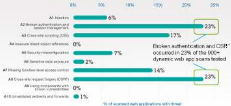
Figure 1. Common vulnerabilities found occurring in web applications tested by the IBM Guard Application Security Management (GASM) service, compared to the OWASP Top 10 for 2013
