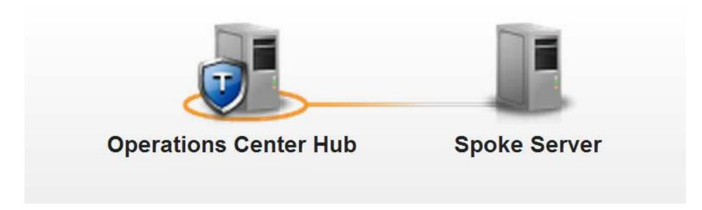
• Hub and spoke servers must have TSM V6.3.4 or later installed.
