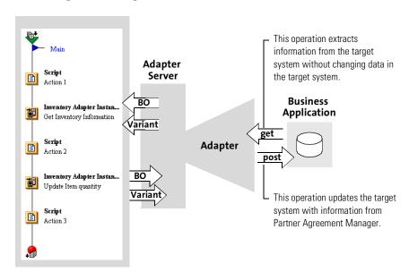
Post operations are stateful, and Get operations are usually stateless. For example, a Get operation extracts information from the target system without modifying the target system's data. A database query is an example of a Get operation. In contrast, a Post operation updates the target system. For example, a Post operation can create a new sales order in a purchasing system.
