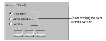
The time-out specifies how long an event remains valid. In other words, the Process Manager has that amount of time to start a public process. Realize that if a public process is suspended, the Process Manager will not start this public process until it is resumed; so if the process is resumed before the event time-out, the Process Manager can start the process.
