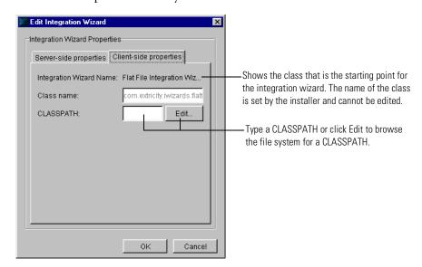
4 Type a CLASSPATH, or click the Edit button to compose the CLASSPATH. The Edit Integration Wizard CLASSPATH dialog box appears. You can use it to build a CLASSPATH by browsing the file system on the client-side computer and selecting directories or archives. You can also type a CLASSPATH.
