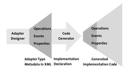
A single adapter type can have more than one implementation. For example, you might want to create one implementation for an in-memory test adapter, and another implementation—the real production version—that accesses a database. Or, you might want to create different implementations for different versions of the production adapter.
