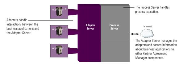
Adapters handle interactions between the external business applications and the Adapter Server. The Adapter Server, in turn, manages the adapters and serves as a conduit for configuration and other information about external business applications. The Adapter Server also ensures consistent handling of state management and audit capture within a process.
