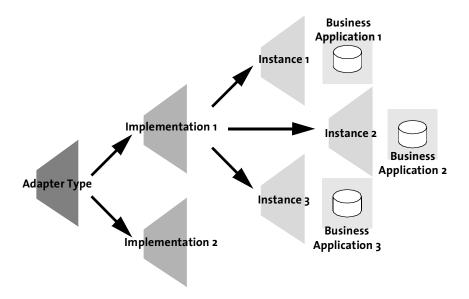
The adapter type, which is stored in XML format for import and export, contains adapter information, including what operations, events, and properties the adapter has. You specify this information in the Create Adapter Type dialog box in the Adapter Designer. For example, these are the properties defined in the adapter type for the example purchasing adapter.
