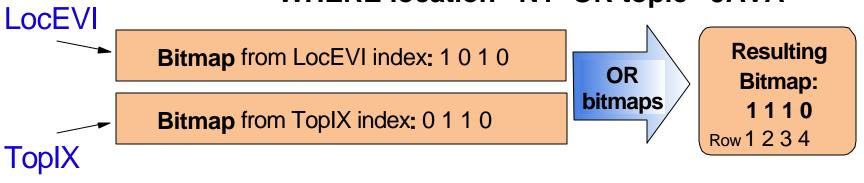
Bitmaps can be derived from binary radix or <u>encoded vector indices</u>
