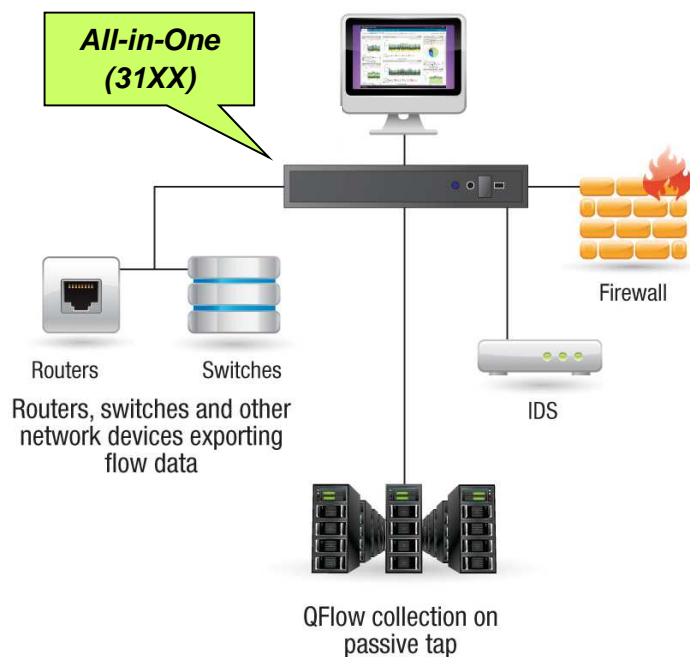
Sample IBM Security QRadar SIEM all-in-one deployment QRadar web console
