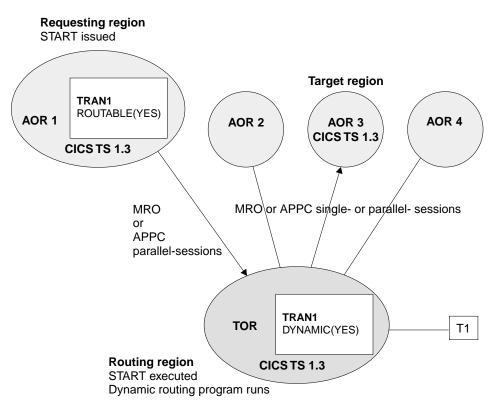
Figure 10. Dynamic routing of a terminal-related START command issued in an AOR. The requesting region, the TOR, and the target region are all CICS TS Release 3. The requesting region and the TOR are connected by an MRO or APPC parallel-session link. The TOR and the target region are connected by an MRO or APPC (single- or parallel-session) link. The transaction definition in the requesting region specifies ROUTABLE(YES). The transaction definition in the TOR specifies DYNAMIC(YES).
