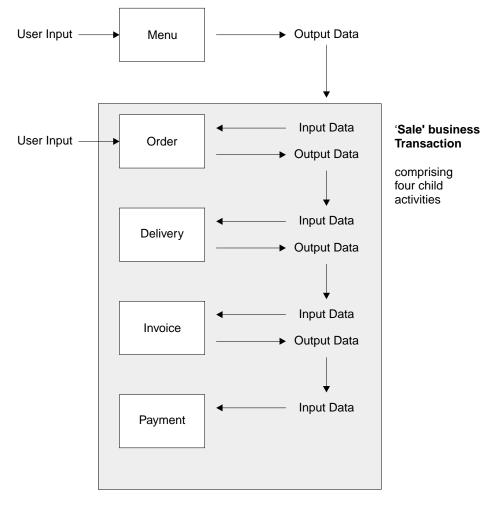
Figure 17. Data flow in the Sale example application. (The root activity is not shown.)
