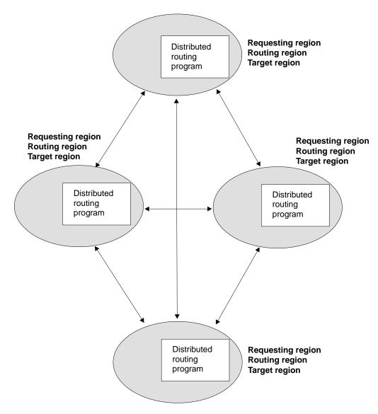
Figure 8. Dynamic routing using a distributed routing model. Each region may be both a routing region and a target region.
