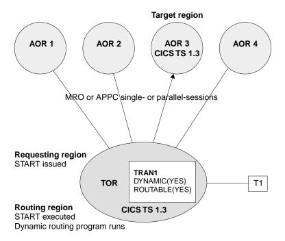
Figure 12. Dynamic routing of a terminal-related START command issued in a TOR. The TOR and the target region are both CICS TS Release 3. The TOR and the target region are connected by an MRO or APPC (single- or parallel-session) link. The transaction definition in the TOR specifies both DYNAMIC(YES) and ROUTABLE(YES).
