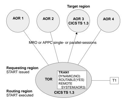
Figure 11. Static routing of a terminal-related START command issued in a TOR, using the enhanced method. The TOR and the target region are both CICS TS Release 3. The TOR and the target region are connected by an MRO or APPC (single- or parallel-session) link. The transaction definition in the TOR specifies DYNAMIC(NO) and ROUTABLE(YES). The REMOTESYSTEM option names the AOR to which the transaction is to be routed.
