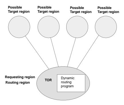
Figure 7. Dynamic routing using a hub routing model. One routing region (the TOR) selects between several target regions.
