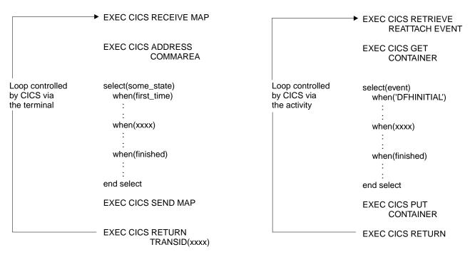
Figure 16. Comparison between a terminal-related pseudoconversation and a BTS activity that is activated multiple times
