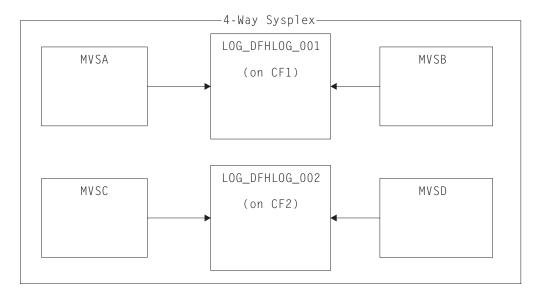
Figure 9. Sharing system logger structures between MVS images
