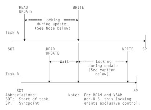
Figure 13. Locking during updates to nonrecoverable files. This figure illustrates two tasks updating the same record or control interval. Task A is given a lock on the record or control interval between the READ UPDATE and WRITE commands. During this period, task B waits.
