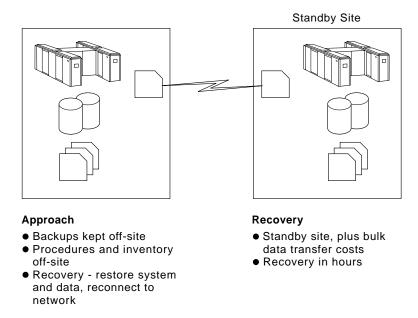
Figure 44. Disaster recovery tier 3: electronic vaulting
