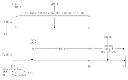
Figure 14. Locking (enqueuing on a resource) during updates to recoverable files. This figure illustrates two tasks updating the same record or control interval. Task A is given an exclusive lock on the record until the update is committed (at the end of the UOW). During this period, task B waits.
