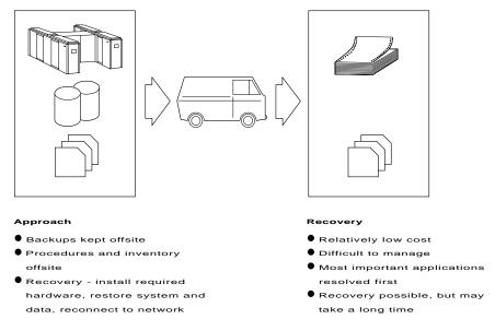
Figure 42. Disaster recovery tier 1: physical removal
