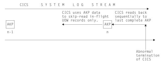
Figure 10. System log scan during restart
