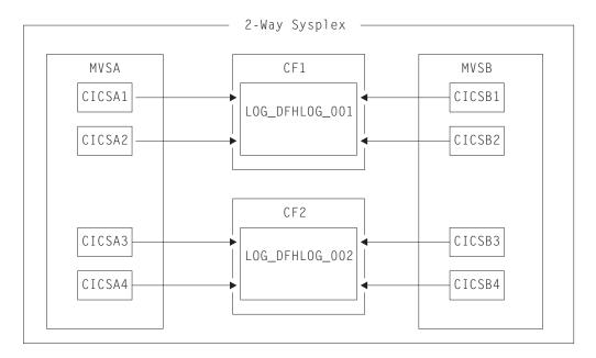
Figure 8. Sharing system logger structures between MVS images
