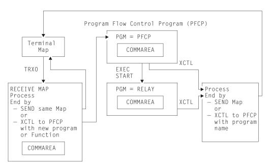
Figure 29. Table-controlled program flow
