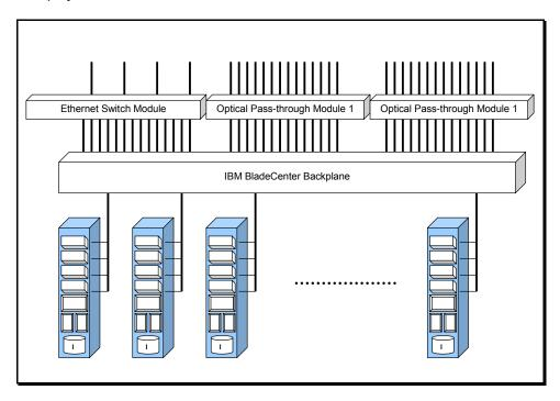
The OPM passes through all ports from all Fiber Channel Expansion cards and enables 4 Gb/s IO over the two FCP2 ports per blade. In a conservative sizing, this would allow up to 300 MB/s sustained storage communication per blade, assuming there is enough disk and controller capacity available on the actual physical storage unit to sustain this level of communications.
