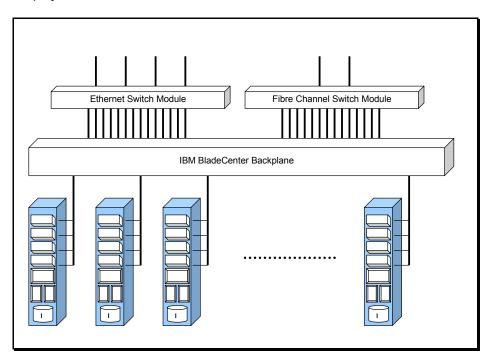
While the backplane adds the functionality to the BladeCenter configuration, and really is the primary differentiator from typical rack-mounted servers (also know as "pizza box" servers) it introduces design considerations that need to be taken into account when designing an overall database cluster for the BladeCenter. However, with the right selection of interfaces and use of standard expansion cards, these considerations do not limit the deployment of the database at all.
