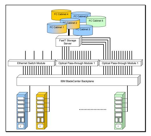
The configuration presented in the diagram enables failover between the two OPMs, redundant paths to the disk cabinets and flexible allocation of the actual disks with the blades. Taking things to the highest level of redundancy, one would deploy a redundant storage system with a redundant BladeCenter for disaster recovery.
