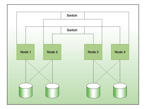
In the mutual takeover case, envision a cluster of N nodes as N/2 pairs of nodes. Node number n is responsible for failover support of node number n+1 (and vice versa), node number n+2 is responsible for failover support of node number n+3 (and vice versa), and so on until you reach the Nth node. Note that this scenario requires that N be an even number.
