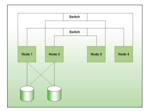
This case relies on a pair+N cluster nodes, where N equals two in this example. Essentially this is the default cluster topology configured by the regdb2udb script. The number of physical nodes in the cluster is a pair+N, where N can be 0 to 6 and is limited by the number of nodes supported by the Sun Cluster 3.x. The prime advantage of this configuration is that the environment is fully redundant; up to N + 1 node failures (given no double
