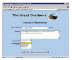
PowerHouse Web enables PowerHouse applications to be accessed from any standard Web browser using an intuitive native HTML user interface. No special plug-ins, ActiveX controls, or Java applets need to be installed or downloaded to the browser.
