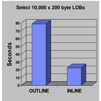
Very small LOBs select, insert shows Up to 70% elapsed time reduction with INLINE LOBs
