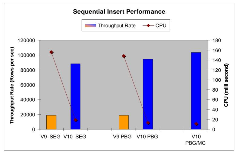
Sequential key insert into 3 tables from JDBC 240 clients in two way data sharing members. Using Multi Row Insert (batch size 100). Each member resides on LPARs with z10 8CPs.
