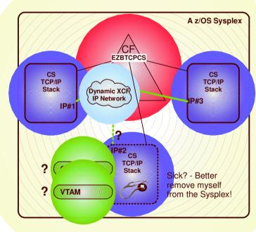
Monitoring is always done, but configuration controls in the TCPIP Profile determine if the TCPIP stack will remove itself from the sysplex.
