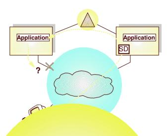
If a network outage condition is detected, the stack may remove itself from the Sysplex if requested by the configuration - allowing backup stacks in the Sysplex to take over its Sysplex responsibilities.
