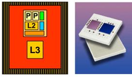
Dual-Core Module POWER5+ Dual-Core chip + L3 cache chip (505, 510, 520, 550, 570) Two processor cores
