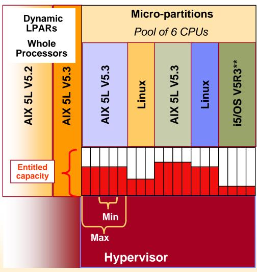
Micro-Partitioning technology allows each processor to be subdivided into as many as 10 "virtual servers", helping to consolidate UNIX® and Linux applications.
