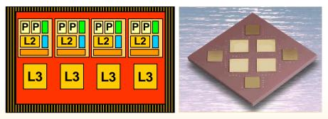
Multi-Chip Module Four Dual-Core POWER5+ chips + four L3 cache chips (590, 595) Eight processor cores
