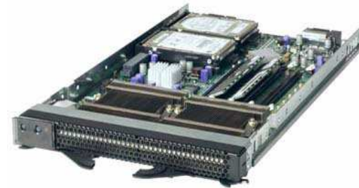
IBM Blade ready for insertion into the BladeCenter
