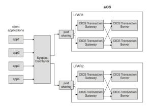
CICS Transaction Gateway for z/OS V8.0, the premium CICS Transaction Gateway product, offers new improvements made to the high availability support introduced in previous versions. For the first time, it is possible to create a sysplex-wide highly available Gateway solution incorporating XA transactions, maintaining transactional scope with CICS systems across the parallel sysplex whilst ensuring that confidence in system uptime is maximized.
