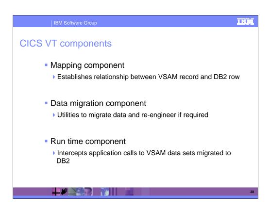
Here's how CICS VT actually works. The tool consists of 3 components:
