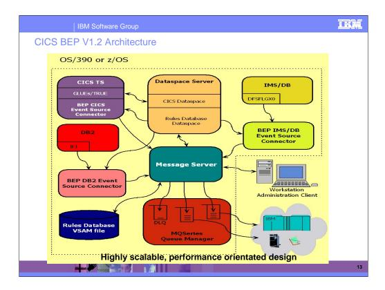
This diagram is the "minimum" configuration for using CICS BEP. In addition to this configuration, the message server can receive messages from multiple event sources, and can put messages to multiple MQSeries queue managers.
