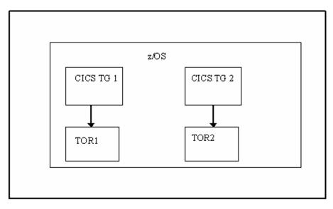
If a TOR fails, the DFHXCURM exit would be expected to substitute the name of the TOR which is still running. The result is the same, but your configuration is more complex:
