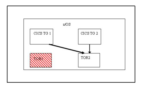
Of course, you could start out with each CICS TG instance connected to a different TOR as in this configuration.
