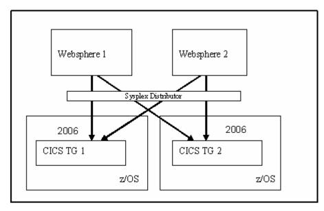
The session set-up between WebSphere Application Server and the CICS TG instances takes place just as in the single LPAR example. Before the connection request is passed through to the TCP/IP stack on a given z/OS LPAR, Sysplex Distributor will choose which of the participating hosts will be the target of
