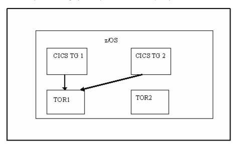
If the TOR abends, the EXCI pipes from the CICS TG are disconnected. When the CICS TG dispatches work to a worker thread and it attempts to send the ECIRequest to CICS, the CICS TG will discover that the pipe is gone. It will then attempt to re-allocate the pipe.
