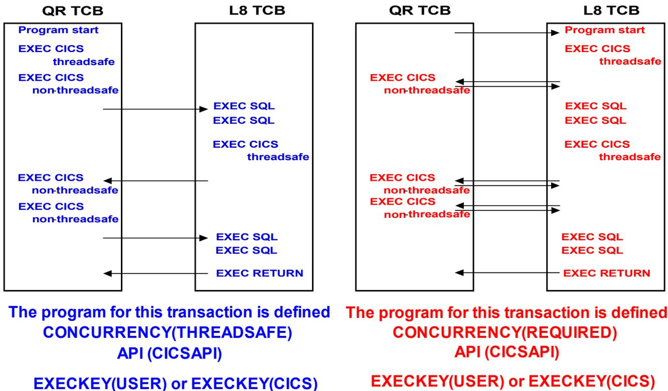
Figure 2. Comparison of CONCURRENCY(THREADSAFE) and CONCURRENCY(REQUIRED)
