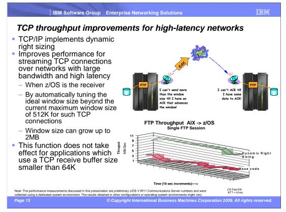
Streaming workload over large bandwidth and high latency networks (such as satellite links) is typically constrained by the TCP window size. The problem is that it takes time to send data over such a network. At any point in time, data filling the full window size is 'in-transit' and cannot be acknowledged until it starts arriving at the receiver side. The sender can send up to the window size and then must wait for an ACK to advance the window before the next chunk can be sent.
