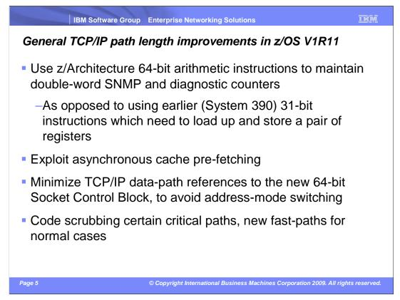
The strategy for Communications Server path length reduction is to reduce memory access latency. Solutions include using newer z/Architecture instructions for maintaining double-word SNMP counters, exploiting a cache-line pre-fetch facility in System z hardware, and minimizing the number of 64-bit socket control block references made along the TCP/IP data path. Some code scrubbing was also done, although V1R10 had already removed much of the low-hanging fruit from the mainline paths.
