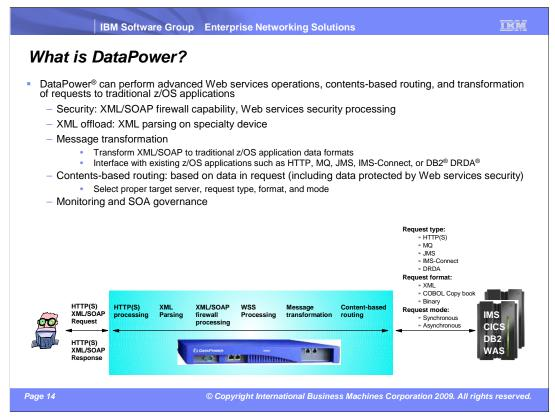
DataPower can be used to provide Web services access to other platforms, such as z/OS.
