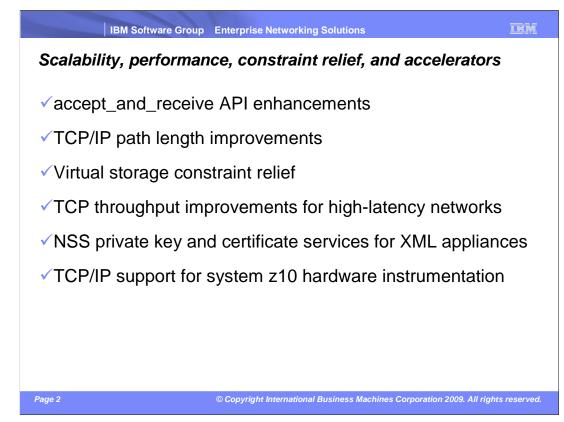
The new asynchronous version of the accept\_and\_receive sockets API is targeting highvolume servers on z/OS, such as WebSphere Application Server. Such servers repetitively issue three sockets calls for every new connection. This enhancement collapses those three sockets API crossings into one thereby saving processor resources and improving response time.
