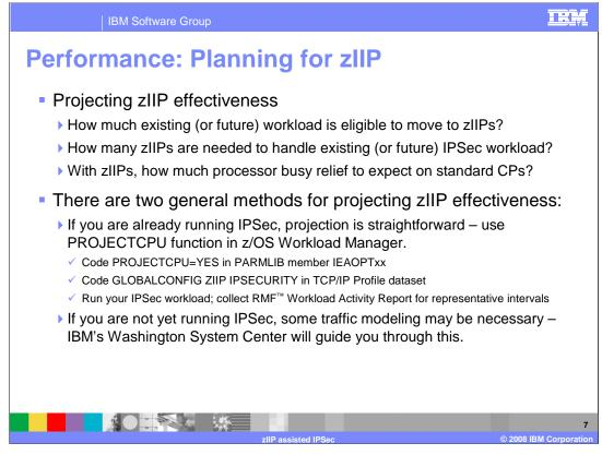
If you are running IPSec, zIIP may significantly reduce the processor utilization of your standard CPs. In planning for zIIP, you need to determine (a) how much of your workload is eligible to move to zIIP, (b) how many zIIPs are required to fully handle that load, then (c) once you do have zIIPs, how much processor busy relief you can expect on your standard CPs.
