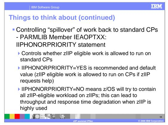
Specifying IIPHONORPRIORITY=YES allows zIIP eligible workload to run on standard CPs, if zIIP work is not completed in a reasonable time period. This is the default and recommended value.
