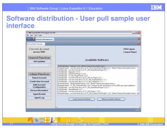
An API is provided to enable applications running on the device agent run-time to get information from the server about what software is available for distribution. The API also enables the application to select one of these bundles to be distributed to the client, along with any required pre-requisites.
