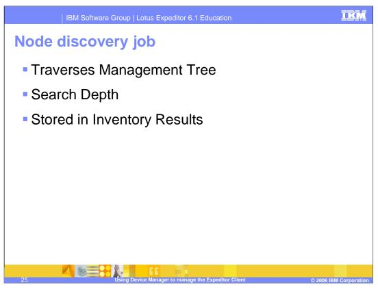
A node discovery job recursively finds sub-nodes on the target devices based upon a target URI.
