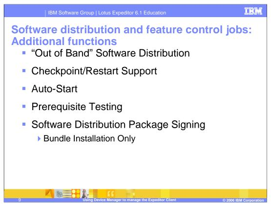
Device Manager uses "out of band" software distribution, which means all file transfers occur directly between the client and the package server using HTTP or HTTPS. This frees up the management server to perform other work.
