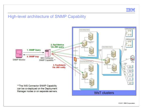
High-level architecture of IP Multimedia Subsystem Connector SNMP Capability is shown in the diagram.
