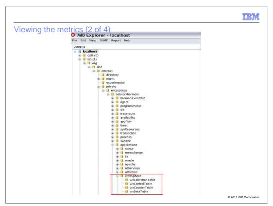
Each MIB describes the hierarchical structure and this screen capture shows the table structure for WebSphere.
