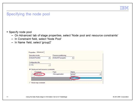
The first method to specify the pool to use is to define a node pool in the configuration file. In the previous example, the node pool for Data Rules stage used group2. On the Advanced tab of the connector properties, select that node pool. The connector will then only run the job on the nodes that are members of that node pool.
