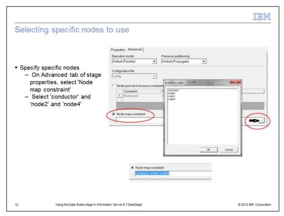
The second method is to have the connector only run on specific nodes. To do this, go to the Advanced tab of the connector properties and select the specific nodes that you want the connector to run.
