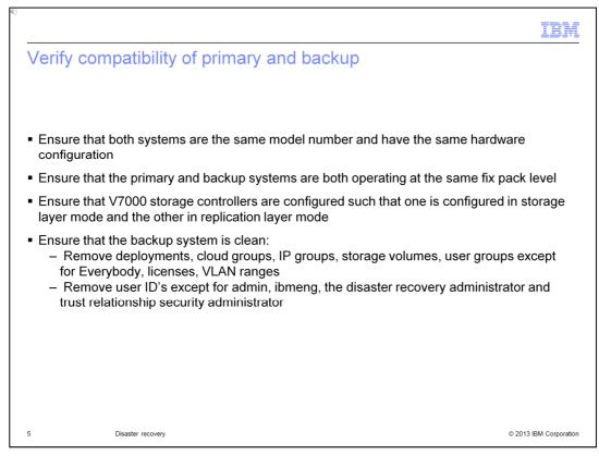
The primary rack and the backup rack must be compatible in a disaster recovery environment. There is a verification function in the user interface so you can perform these checks. Also, when you enable the disaster recovery profiles there is automatic verification with error messages for any failures.
