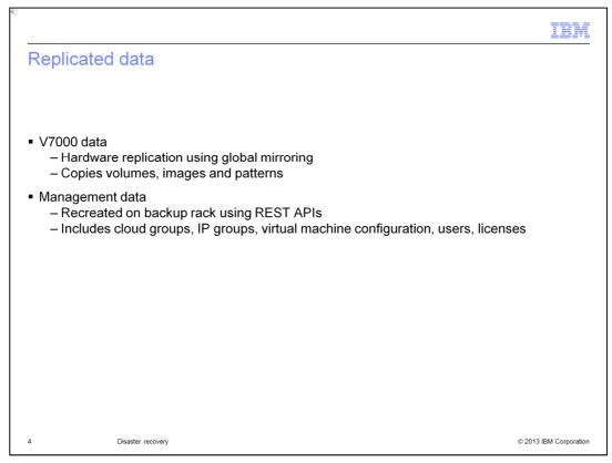
The V7000 storage unit uses global mirroring to make asynchronous copies of your disk. This means that the write is considered complete after it is complete at the local disk. It does not wait for the write to be confirmed at the remote cluster.
