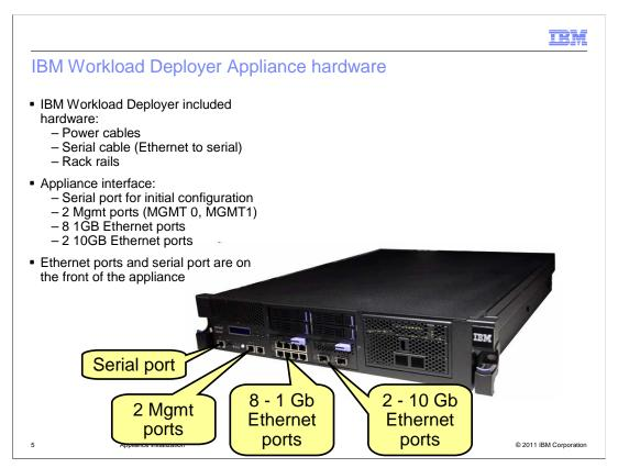
The IBM Workload Deployer Appliance has all the required hardware included with it to install onto the rack, including two power cables, a serial interface connection cable, and rack rails. On the front, from left to right, you have one serial port, two MGMT ports (MGMT 0 and MGMT 1), eight one-gigabit Ethernet ports, and two ten-gigabit Ethernet ports.
