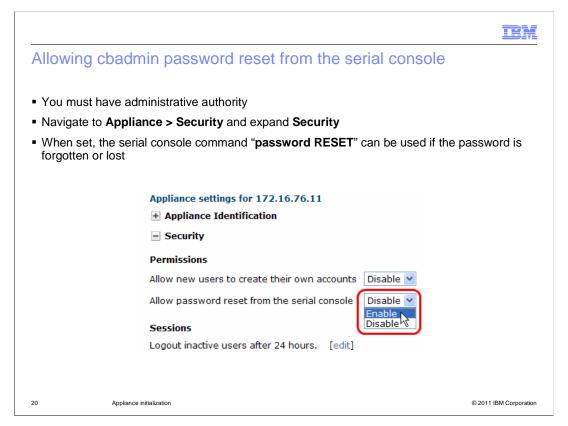
This feature allows you to reset the cbadmin password from the serial console in case you have lost or forgotten the password. Once the "Allow password reset from the serial console" is enabled, then you issue the "password RESET" command in the serial console and you are prompted to type in a new password.
