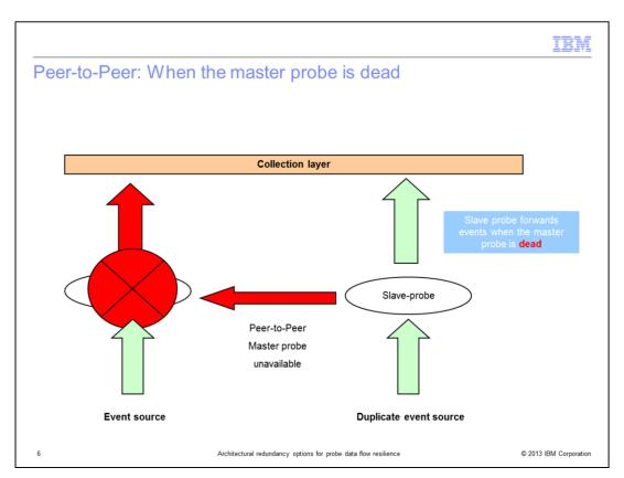
When the master probe is shutdown, the slave probe is unable to check its status with the Peerport. The slave probe then forwards the events it has stored, since the last successful check of the master probe, to the object server it is connected to.
