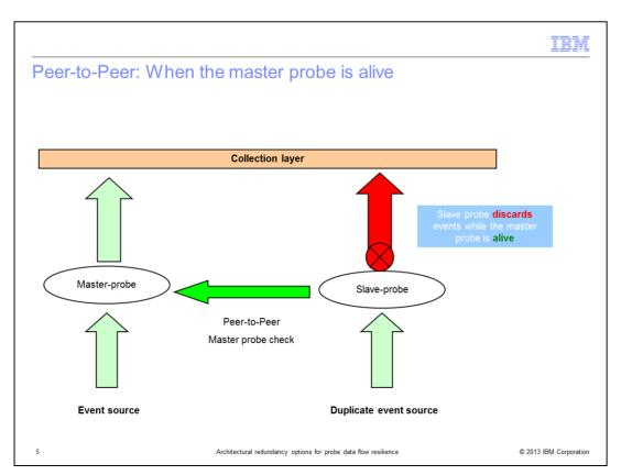
Under normal circumstances, the slave probe checks that the master probe is available by using the Peerport. When the master probe is available, the slave probe discards all of the events it receives.
